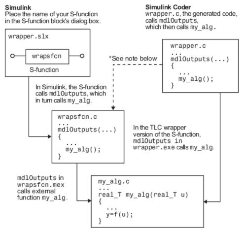
\*The dotted line is the path taken if the S-function does not have a TLC wrapper file. If there is no TLC wrapper file, the generated code calls md10utputs.
