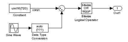
The code generated for the bit-wise operator block reuses a temporary variable that is set up for the output of the sum block to save memory. This results in one very efficient line of code, as seen here.
